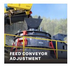
Every product is unique - adjust your product feed trajectory by easily adjusting your conveyor head pulley position.
