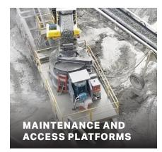
**Full plant access** with 360-degree platforms surrounding the impactor. Safe tread ladder with handrails.
