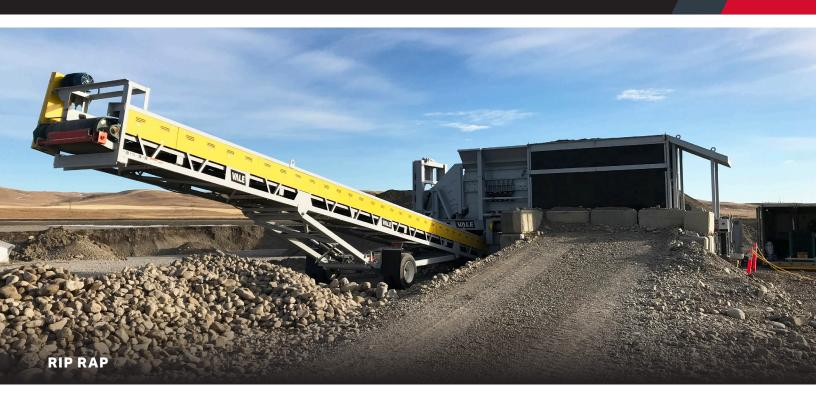
Vale Rip Rap Plants are built with up to 1" thick hopper walls and heavy 3/4" thick chutes to take the abuse. Designed and built with up to a two-stage VGF to most efficiently manage your downstream feeds.
