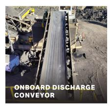
Fold out or raise the discharge conveyor to **reach into screens or feeders** without the need for off-plant conveyors.
