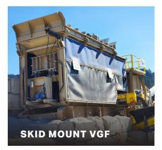
Skid Lift cylinders make the jump from Chassis to Trailer a **safe and simple** process. Feeders may need to be removed to meet transport weights.
