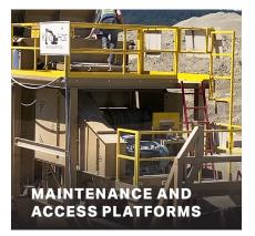
Large upper and lower Jaw platforms that provide **full maintenance access** around the Jaw itself and the Jaw drive components.
