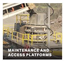
Full plant access with 360-degree platforms surrounding cone. **Cone viewing platform** and metal detector retrieval platform.
