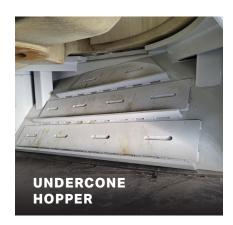
Built for Wear: growser bar rockshelves and heavy AR liners **extend the life** of the hopper. Complete with large access doors.
