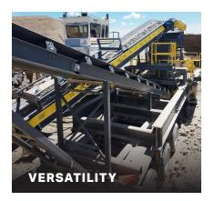
Configurable as Rear Feed/Rear Discharge or Rear Feed/Side Discharge, with left or right-hand orientations.
