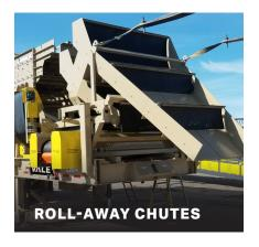
Simplify media changes and maintenance with the roll-away chute assembly, **giving you full access** to all screen decks from both ends.
