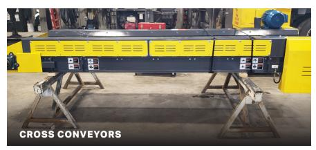
Fully enclosed cross conveyors to remove bypass or sized products while keeping errant rocks out of the belts.
