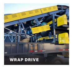
Plenty of power to load up the overhead feed belt to feed a larger screen and **increase your throughput.**
